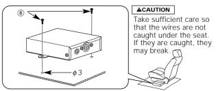
Install the FM modulator unit beneath the front seat using Metal fixture and Bind head screw as shown in the above figure.
