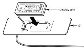
Pass the wire from the display unit through the hole on the trim mount plate and push fit the display unit into the trim mount plate until it locks.
