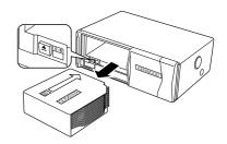
Open the CD changer door, and press the "EJECT" button.
